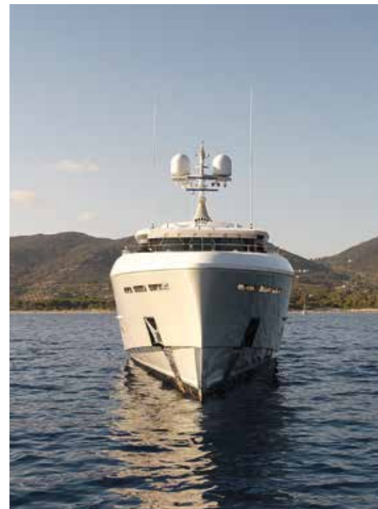
Left: Endeavour II has a range of 5,000 nautical miles thanks to her aluminium hull design and diesel-electric propulsion system, comprising twin Caterpillar C32 Acert engines and a pair of Rolls-Royce azimuthing pods
