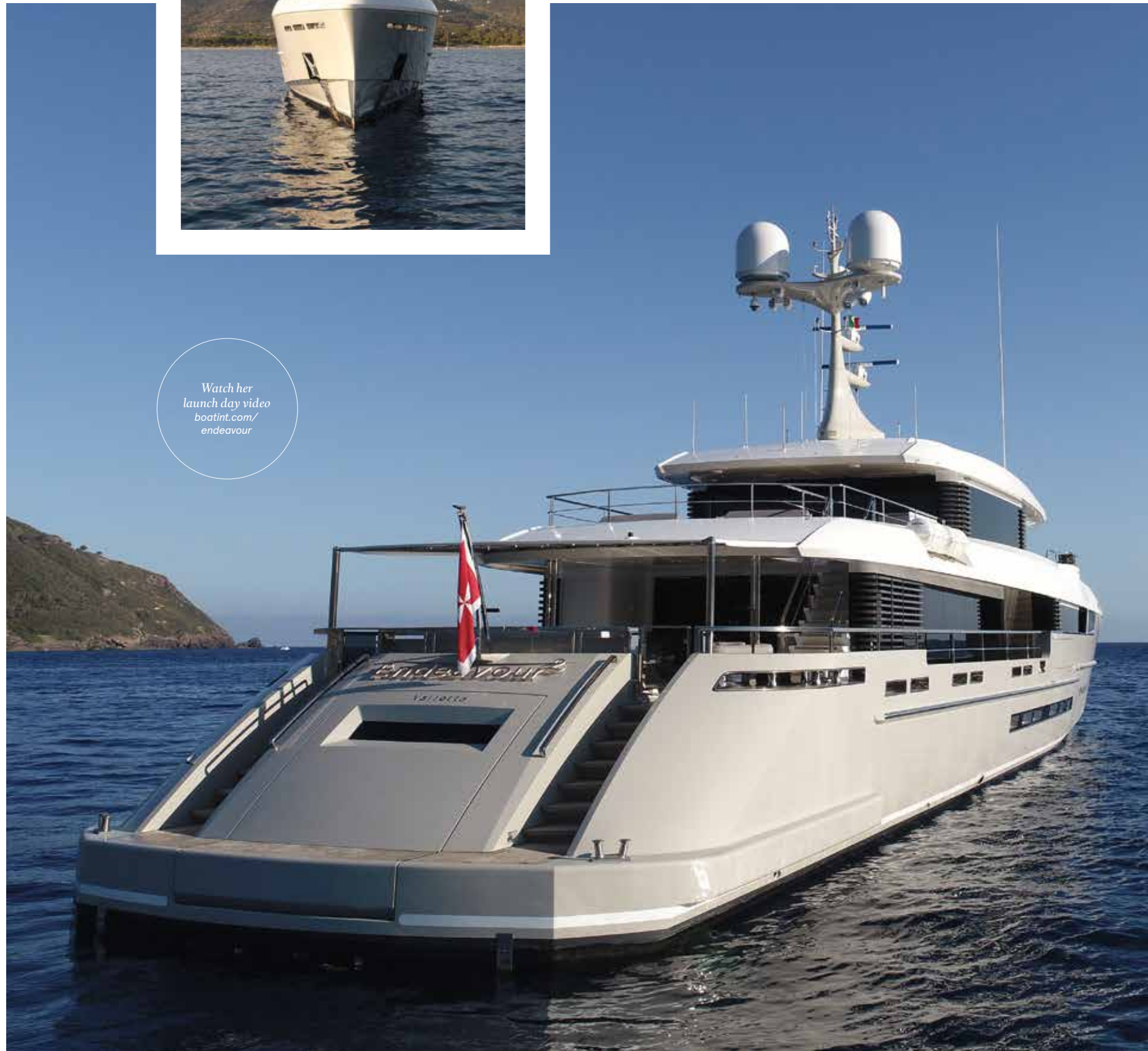
Left: Endeavour II has a range of 5,000 nautical miles thanks to her aluminium hull design and diesel-electric propulsion system, comprising twin Caterpillar C32 Acert engines and a pair of Rolls-Royce azimuthing pods
